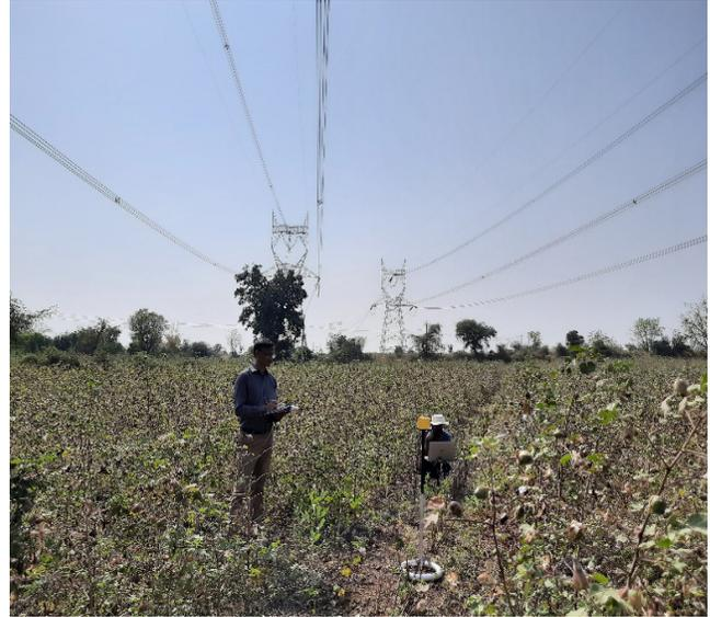
**Figure 1.** EMF measured in 765 kV S/C transmission lines in cotton field.
