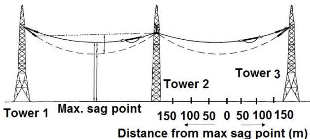
**Figure 5.** Schematic of longitudinal measurement of EMF strength of 765 kV S/C transmission line.
