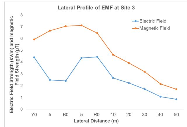
Figure 11. Lateral profile of EMF at site 3.
