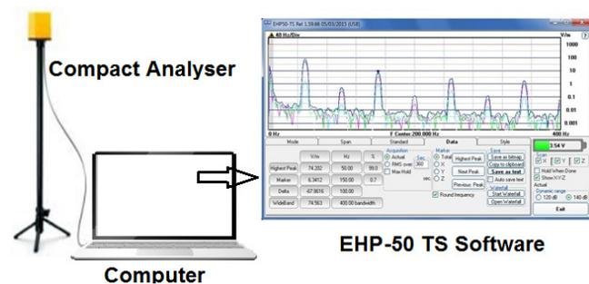
**Figure 6.** EHP-50 Compact Field analyser.
