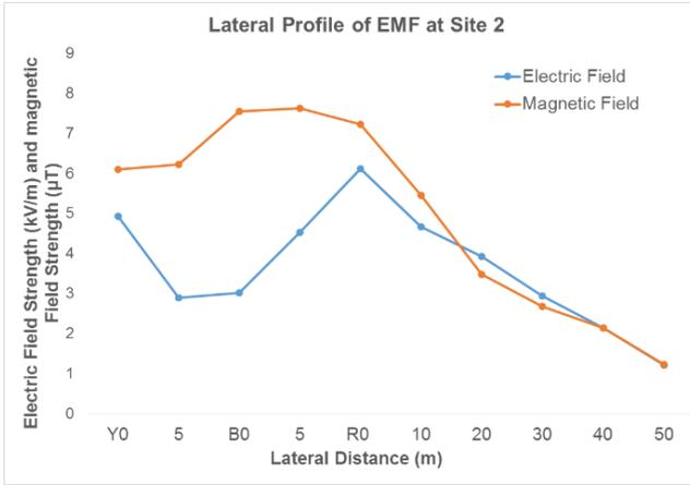
Figure 9. Lateral profile of EMF at site 2.
