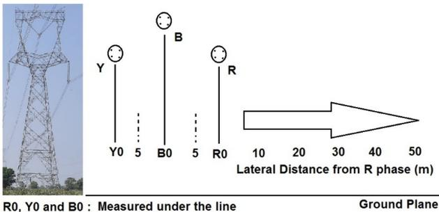
**Figure 4.** Schematic representation of lateral profile of 765 kV S/C transmission line.
