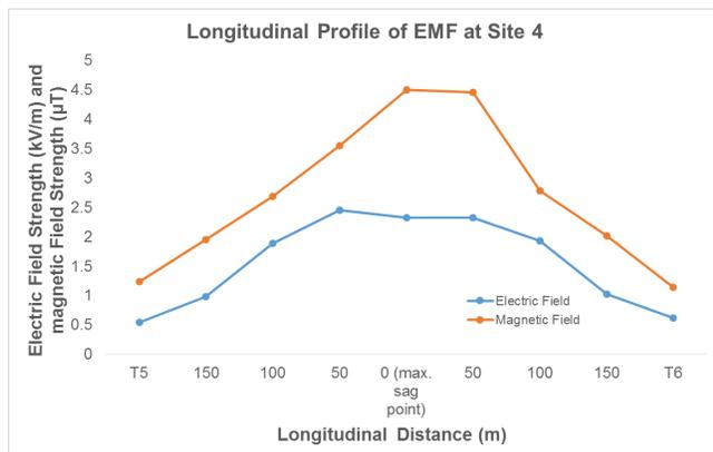
**Figure 14.** Longitudinal profile of EMF at site 4.
