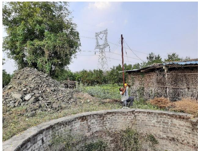
**Figure 3.** EMF measured in 765 kV S/C transmission lines near open well and isolated metal roof shed.
