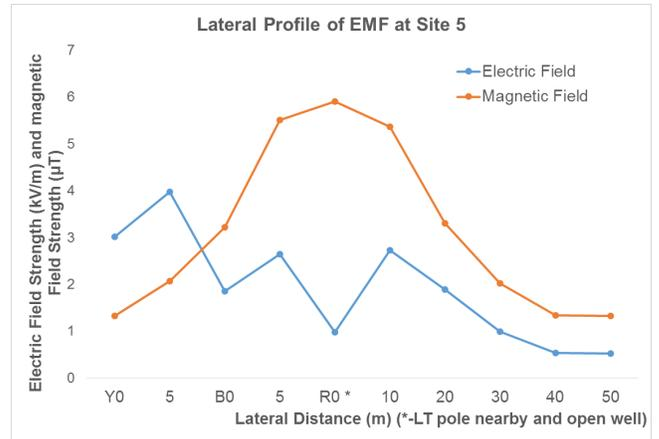
**Figure 15.** Lateral profile of EMF at site 5.
