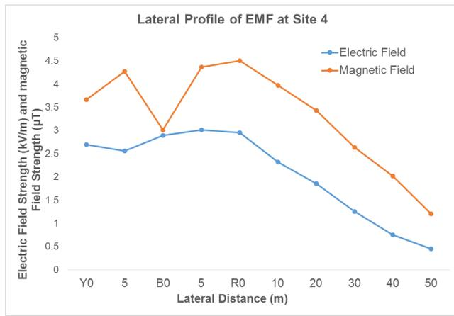
**Figure 13.** Lateral profile of EMF at site 4.
