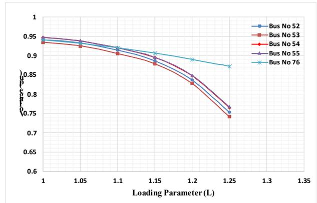
Figure 6. Voltage profile with 40% wind penetration with compensation.
