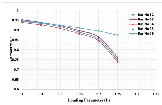
Figure 7. Voltage profile with 50% wind penetration with compensation.
