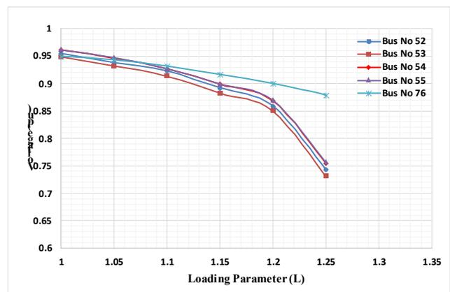
Figure 8. Voltage profile with 60% wind penetration with compensation.
