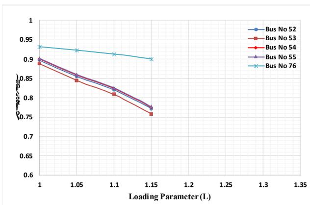
Figure 5. Voltage profile with 60% wind penetration without compensation.
