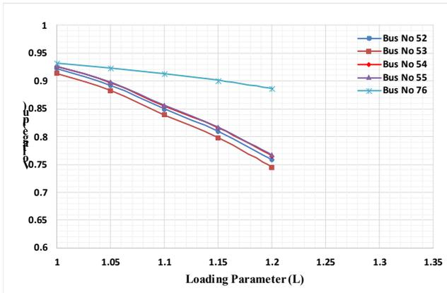
Figure 3. Voltage profile with 40% wind penetration without compensation.
