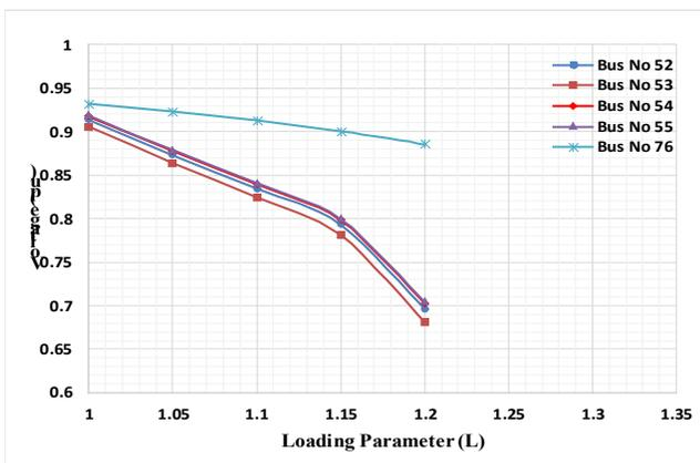
Figure 4. Voltage profile with 50% wind penetration without compensation.
