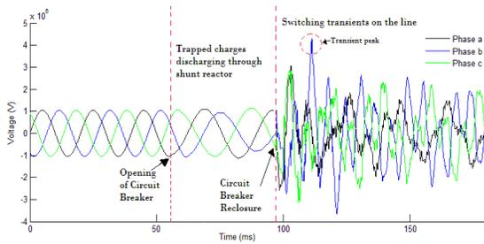
Figure 4 voltages at the receiving end.
