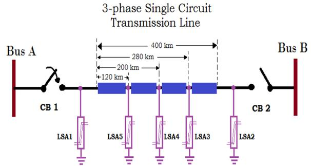
**Figure 8.** A schematic representation of LSA'S placed at different locations along the line.
