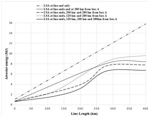
Figure 10. Energy absorbed by the lsa’s placed at various locations.
