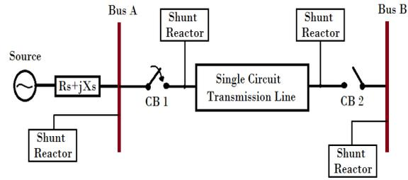
**Figure 1.** Single Line Diagram (SLD) of the uhv system studied.
