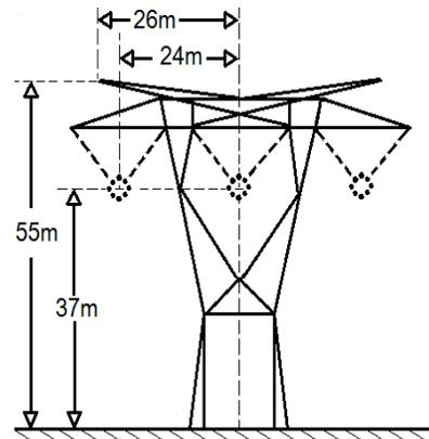
**Figure 2.** Single circuit uhv tower configuration.
