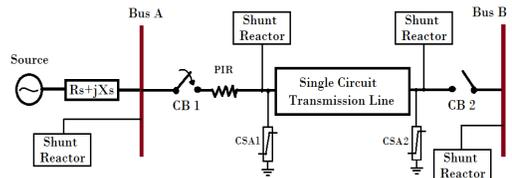
Figure 5. Single line diagram of UHV system with pir protection.
