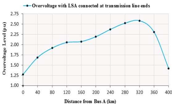
**Figure 7.** Overvoltage profile along the transmission line with lsa's connected at line ends.
