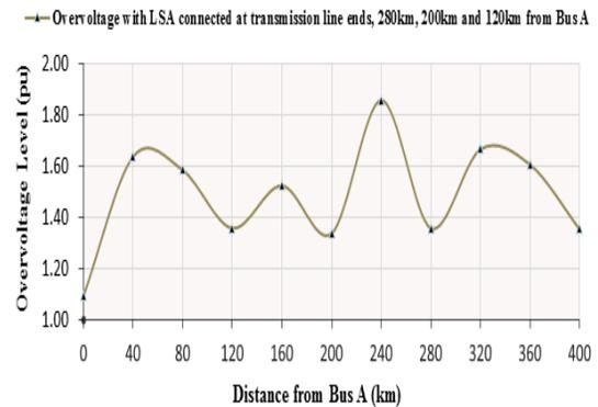
**Figure 9.** Overvoltage profile along the transmission line with lsa's at different locations along the line.
