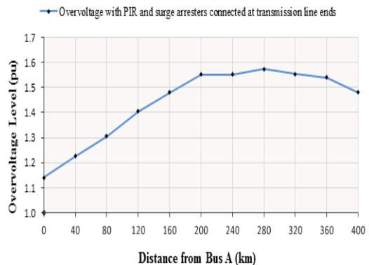
Figure 6. Overvoltage profile along the transmission line with pir and surge arresters.
