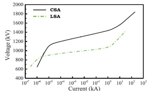
**Figure 3.** Nonlinear V-I characteristics of the Conventional Surge Arrester (CSA) and Line Surge Arrester (LSA).
